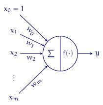
• The unit calculates a weighted sum of the inputs
